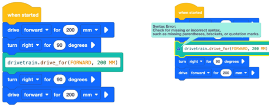
(a) (b) Figure 2: (a) Regular Switch block; (b) Switch block with syntax error warning;
